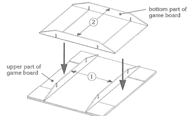
In order to do so you have to put the upper part of the game board face down on the table and fold up the two flaps (1) on the back. Also fold up the flaps of the bottom part (2) of the game board. Now insert these two parts into each other so that they slot together.
